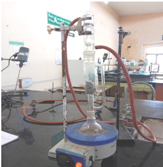
Figure No.4: Hot Maceration Process (Soxhlet Apparatus)
